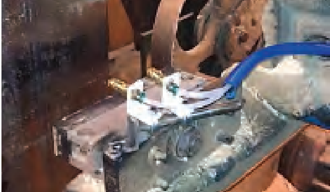
Band saw shown with two nozzles mounted just above guide and two additional nozzles mounted on the inside of the saw. Nozzles can be mounted any place on the inside back that is easy to attach. The objective is to coat the blade before it reaches the top wheel. This prevents pitch transfer to the wheel.
